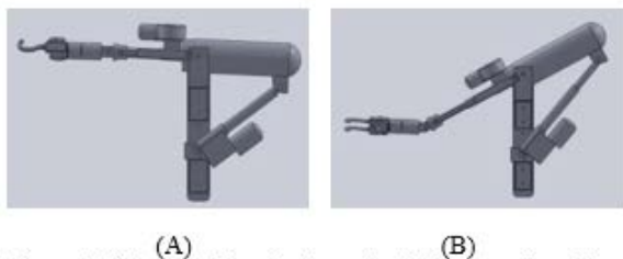
Figure 4. Side view of the robotic arm in (A) the neutral position with no extension or rotation of any motors or actuators, and (B) a position that demonstrates movement of the joints with each joint having partial extension and/or rotation.
