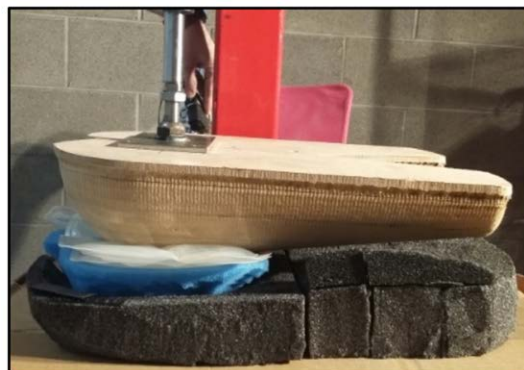
Figure 1: PRCLI attached to a pneumatic testing rig, applying load to a cushion prototype
