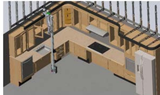
Figure 1. SolidWorks model of the KitchenBot system in the HERL research kitchen. Shown with the initial robotic arm, the JACO, mounted on the column.
