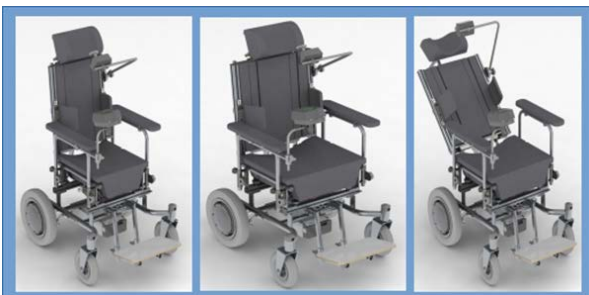
Figure 2: Possibilities of seating adjustments (from left to right): seat and backrest with 36cm of width, seat and backrest with 46cm of width, and backrest angle adjustment.
